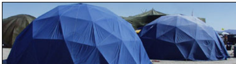
Figure 36: The geodesic dome is a lightweight, but extremely strong, shelter developed by Buckminster Fuller in order to address the post-war housing crisis.
