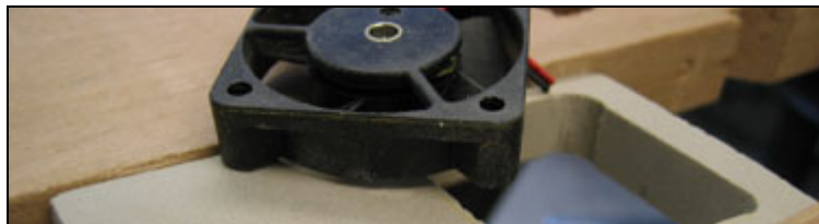
Figure 67: The main parts of the wind music player consist of a small fan and a body of high-density foam.
