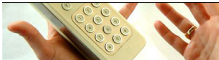
Figure 21: The SoMo1 mobile phone gives the user a electrical shock depending on how loud the person at the other end is talking.
