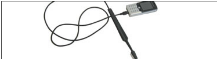
Figure 72: The final version of the toothbrush battery charger mock-up.
